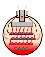
The heat exchanger consists of a steel shell insulated with closed-cell foam material, while the tube bundle is made with copper tubes. The heads can be removed for tube inspection and cleaning. Victaulic couplings on water side (complete with nipple for connection). On the hydraulic connections of the heat exchanger, there are also pipe taps for the differential pressure switch, and wells for the temperature probes.
