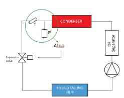
The electronic expansion valve is designed to offer enhanced stability during operation and to maximise the use of evaporation under all load conditions. This also acts as shut-off valve on the liquid line, thereby preventing hazardous refrigerant migrations during compressor stops.
