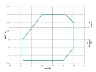
**LWTs:** water outlet temperature from the source-side heat exchanger **LWTu:** water outlet temperature from the user-side heat exchanger **LWTr:** water outlet temperature from the recovery exchanger
